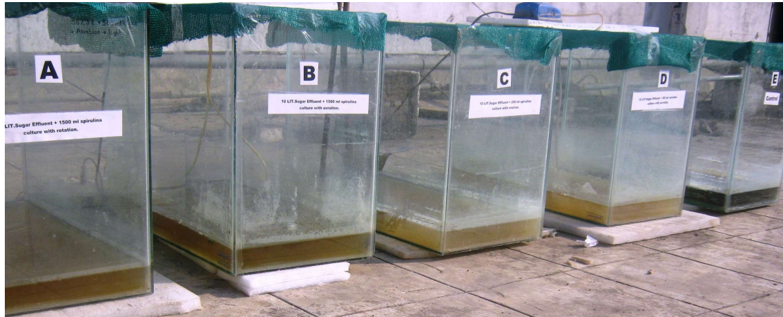
Open type bioreactor for industrial effluent treatment
